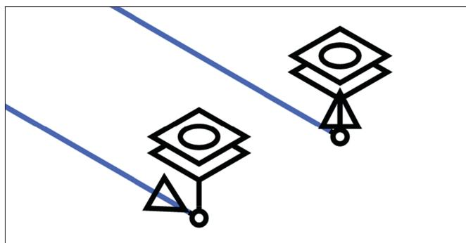
Reductions can be positioned directly after an outlet on vertical or horizontal pipes. This increases accuracy in material lists and reduces manual adjustments in space-constrained layouts.
