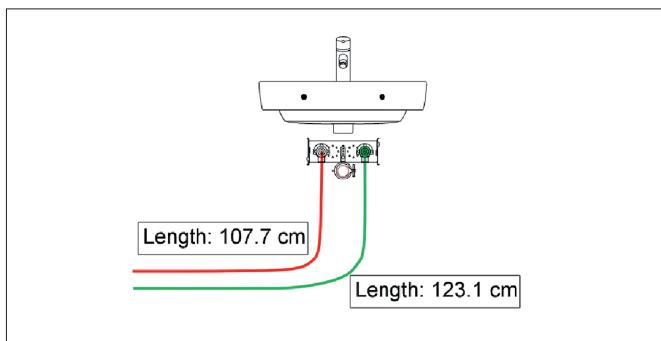
Splines representing bendable pipes can now be dimensioned in 2D elevation drawings, improving workflow efficiency.
