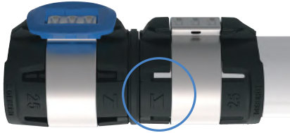
Figure 4: If the insertion depth is correct, the pipe can be seen through both inspection windows.
