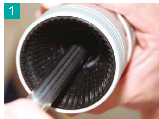
CUT AND DEBURR PIPE
