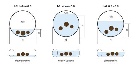
↑ Appropriate size of discharge pipe is crucial for a good self-cleaning of the system.
