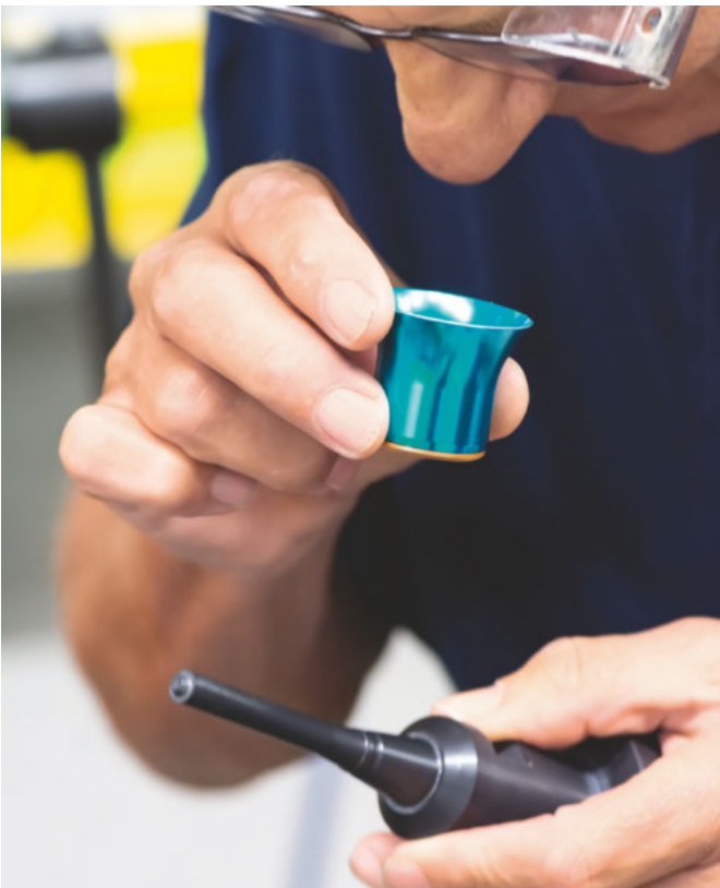
↑ Using an eyepiece, a member of staff checks whether the surface of the mould core is up to scratch.
