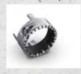
The Geberit fire protection sleeve RS90 Plus prevents fire from spreading via the drainage system. Under the influence of heat, the material in the fire protection sleeve swells, completely compressing the discharge pipe and thereby preventing the fire from spreading to other floors or rooms.
