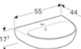
55cm washbasin W 55 / D 44 / H 17.7cm Visible overflow.
