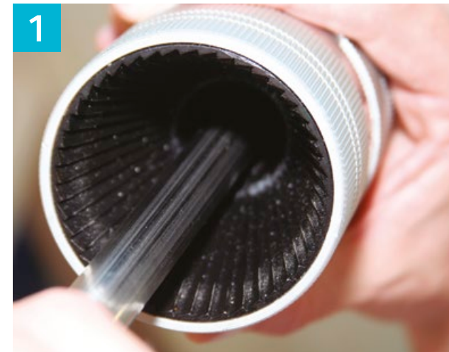
Cut and deburr pipe
