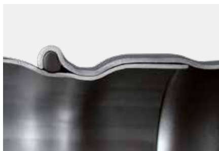
↑ Mechanically stable and hydraulically leakproof: a pressed Mapress joint.
