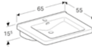
65cm square washbasin, barrier free W 65 / D 55 / H 15.5cm Visible overflow.
