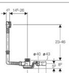
Geberit bath drain with push actuation PushControl
