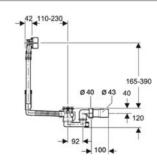
Geberit bath drain with turn handle actuation and inlet
