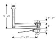
Geberit washbasin connector clou with lever actuation for basins with
