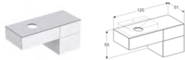
120cm cabinet for lay-on washbasin, with three drawers W 120 / D 51 / H 55cm With integrated shelf surface and trap.
