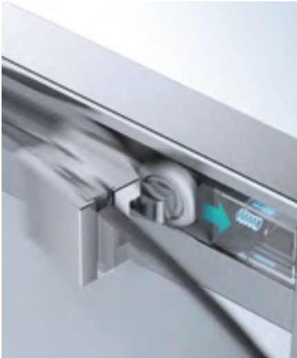
SPRING LOADED BUFFERS Provide an enhanced cushioning effect for improved acoustics when opening and closing the shower door, as well as smoother action when using the shower enclosure.
