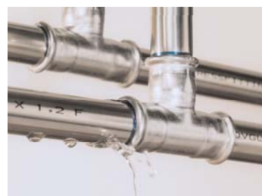
Mapress seal: leaks in unpressed state
